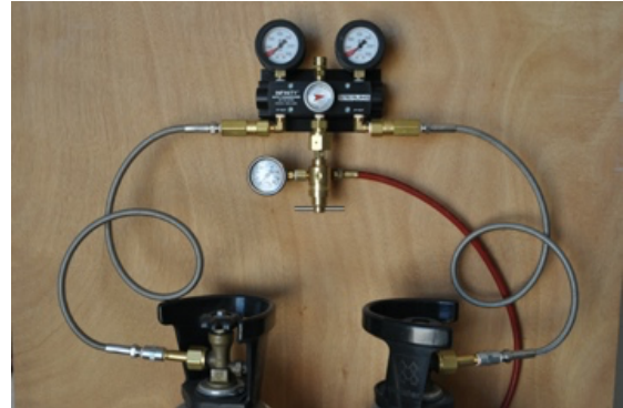
Figure 3 (Right tank set as Priority by Selection Knob, Left Tank is Reserve)
